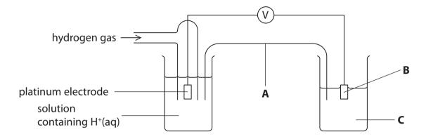
(i) Identify, by name or formula, the substances needed in the salt bridge and the right-hand half-cell to measure the standard electrode potential.
